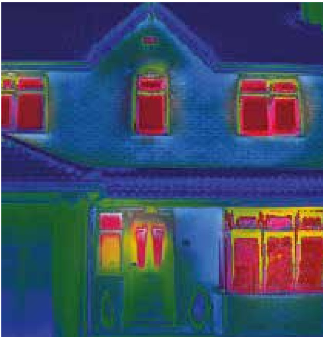
HEAT LOSS FROM A TRADITIONAL WINDOW
